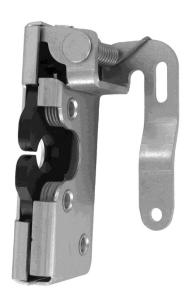
This two rotor latch is a sub-platform to the Tri*Mark* proven 050-0100 series latch and is designed for medium to heavy-duty applications for on or off highway entrance doors, compartments and access panels. It features a coaxial trip mechanism for applications where it is desirable to provide additional support to the trip lever and is FMVSS 206 (ECE R11) compliant.
